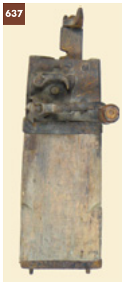
637. Very interesting, blacksmith made, wagon jack. Hollowed out, tapered body is of a heavy, oak-like wood and most, if not all of the metal parts appear to be hand forged. Wide notches on sides presumably for fastening to the wagon. Shaft elevates by turning a hand crank which activates a locking cog. Top of jack shaft clearly marked "1860". Wooden body measures approximately 18" T x 7" W x 3" T (at base). Measures about 32" fully extended. Some surface rust. Good overall condition. 300-450
